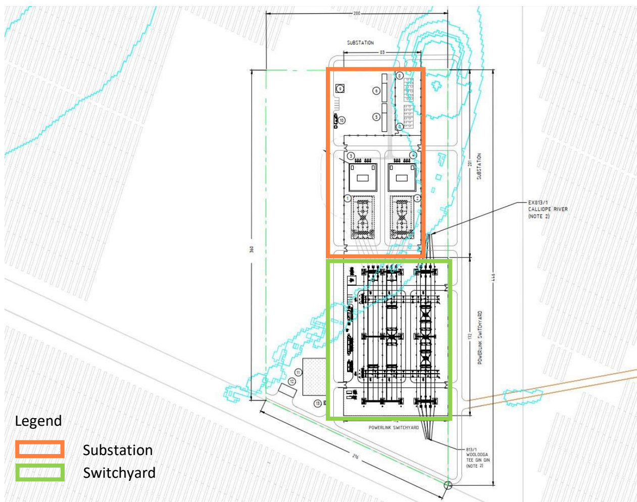
Figure 3-5: Electrical substation layout (Source: QGE Pty Ltd).
